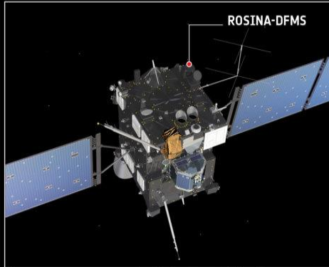
The measurements were made with the Rosetta Orbiter Spectrometer for Ion and Neutral Analysis Double-Focusing Mass Spectrometer (ROSINA-DFMS).
